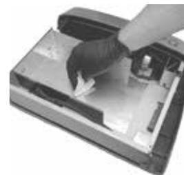
Step 7 - Carefully locate wafer connection “I” into black socket, then firmly push and manipulate until fully inserted.
